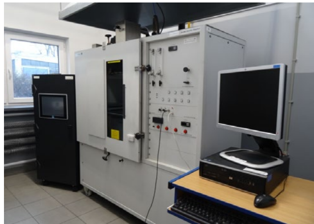
Fig. 1. Smoke chamber according to ISO 5659-2 [11].
