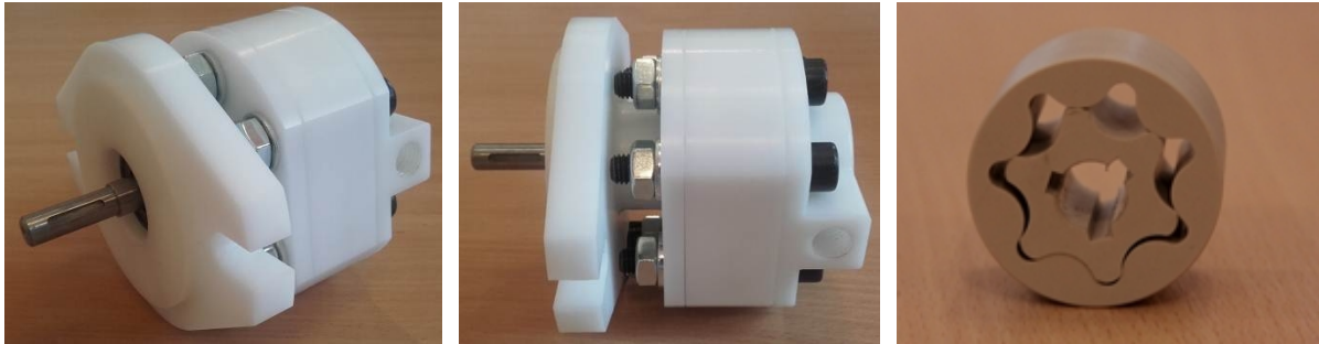
Fig. 4. View of a gerotor pump with a body made of plastics
