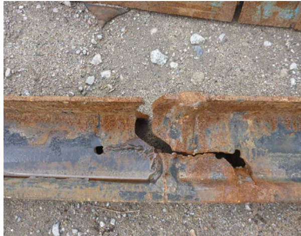
Fig. 5. Example of fracture of a rail joint (a thermite weld) of the 60R2 rail.
