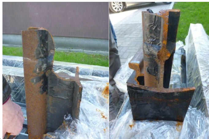
Fig. 2 Cracked 60R2 rail in the area of weld occurrence.
