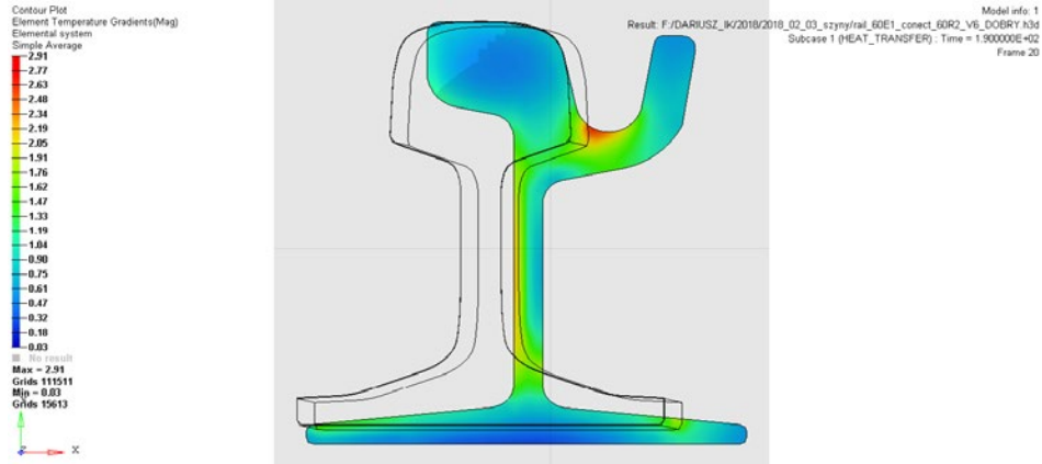
Fig. 8. Temperature gradient in the 60R2 rail, cross section 10 mm away from the joint (thermite weld).
