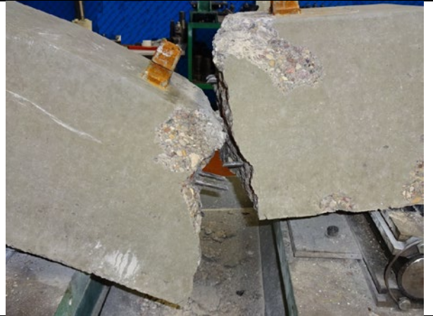
Fig. 8. Fracture of the PS-94 sleeper reinforced with a smooth bar.
