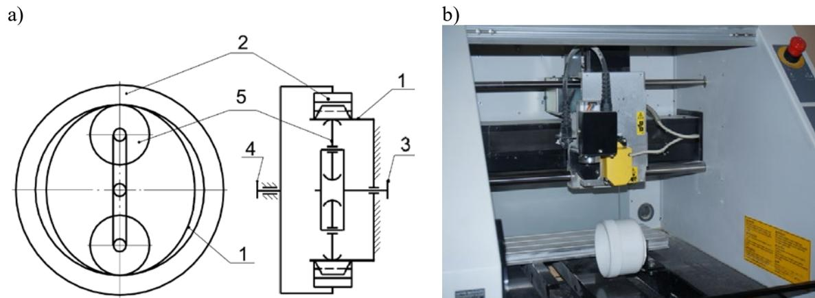
*Fig. 1. Harmonic drive: a) scheme: 1-flexspline, 2-circular spline, 3-input shaft, 4-output shaft, 5-two-roll generator, b) measurement of the profile of the flexspline in a longitudinal section on the Roland MDX-40 cnc milling machine.*
