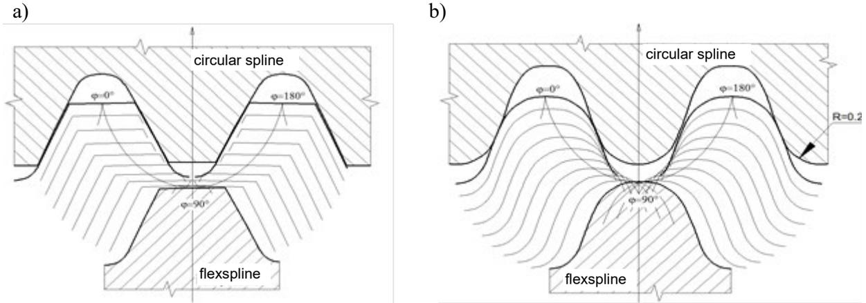
*Fig. 4. Trajectory of the flexspline's tooth: a) for the theoretical outline, b) for the outline of the model obtained by 3D printing method.*
