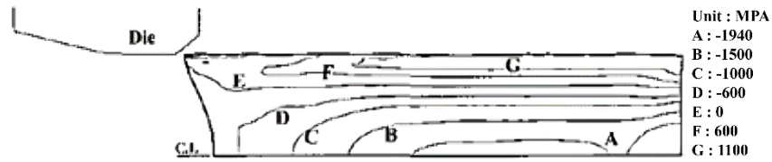
Figure 2: Gradient of residual axial stress after drawing [3].
