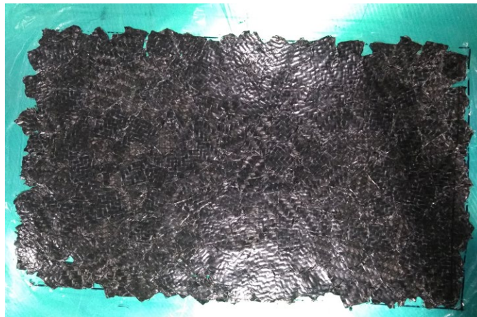
Fig. 1: A sheet of manufactured chip-SMC consisting of 25mm square chips
