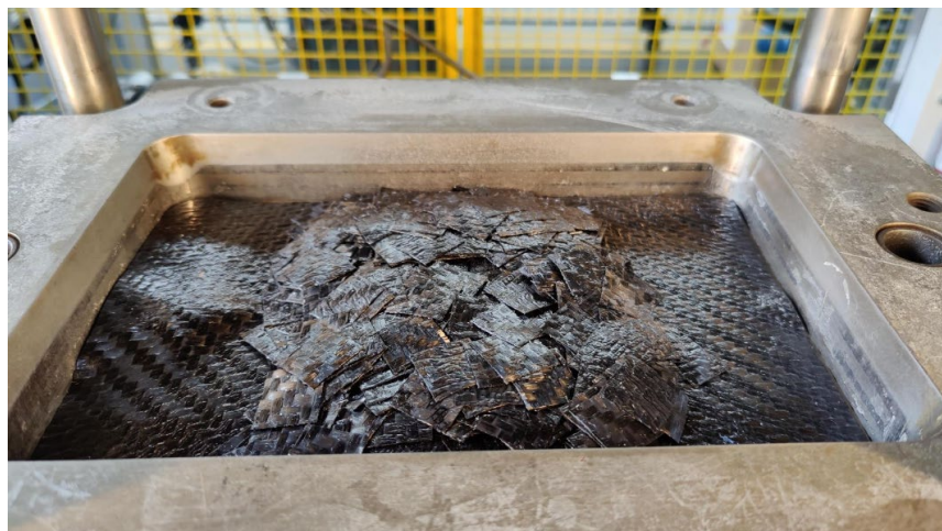
Fig. 8: Prepreg plies and chip-SMC charges in the flat plaque mould cavity on the Langzauner press
