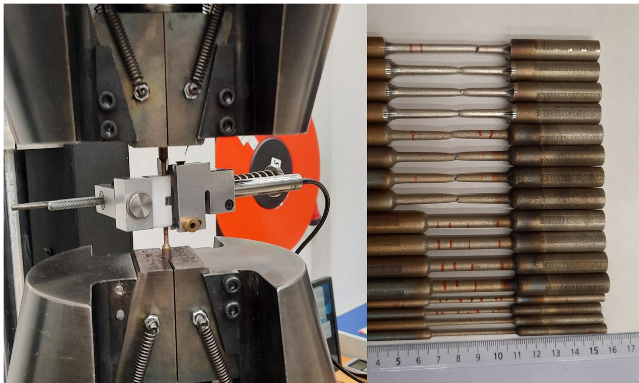
Figure 3. Sample with an extensometer attached and marked samples during testing.
