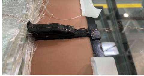
Figure 4: Focus on Sensor integration in the composite part
