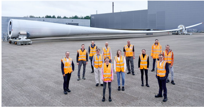
Figure 1: The second 100% recyclable ZEBRA 77m wind blade manufactured by LM Wind Power
