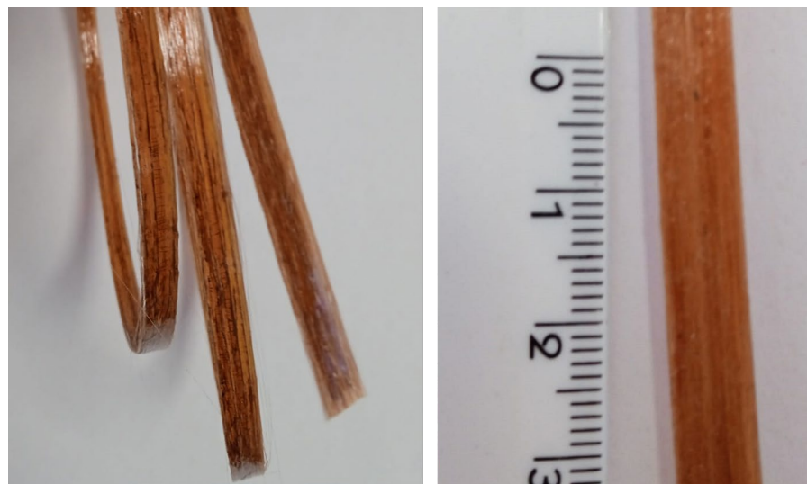
Figure 1. Preconsolidated tapes in glass fiber reinforced recycled PET.
