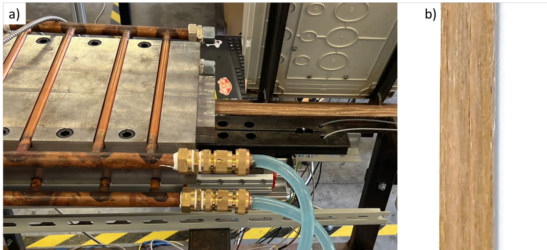
Figure 3. a) Pultruded composite at the cooling die outlet; b) Surface of the pultruded composite.
