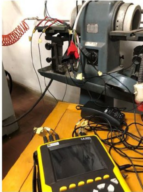
Figure 1. Experimental setup to measure current and tension during FSW process
