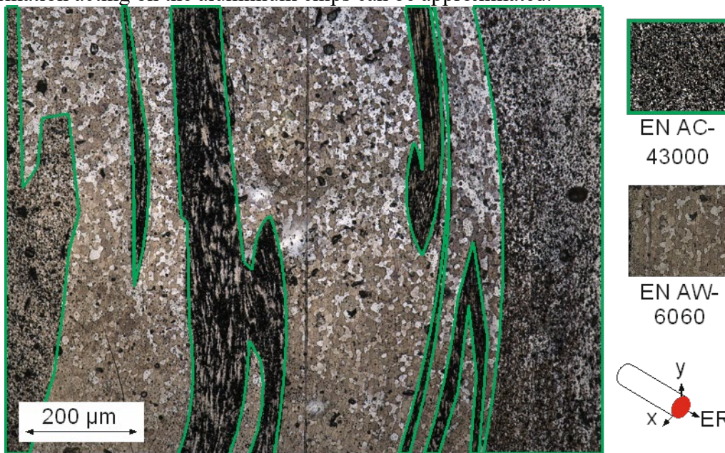
Figure 6: Microstructure of an alloy mixture of 75 % EN AW-6060 and 25 % EN AC-43000
