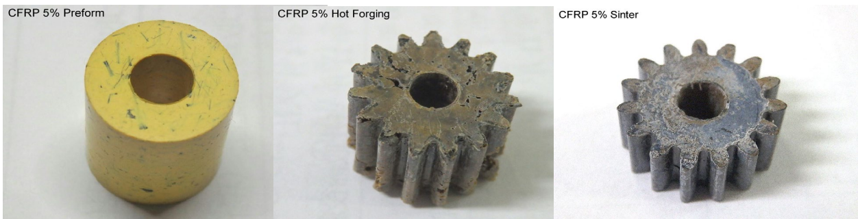
Figure 11. Green compact, hot-forged and sinter-forged gears including the carbon fibers by 5 mass% into polyimide powders.
