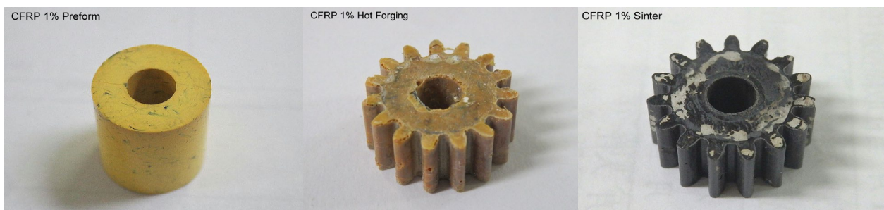
Figure 9. Green compact, hot-forged and sinter-forged gears including the carbon fibers by 1 mass% into polyimide powders. The white colored depots were residual solid lubricants of hBN (hexagonal boron nitride) powders.
