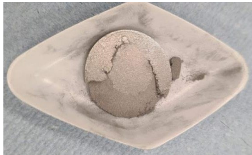
Figure 1: Pre-alloyed NiTi powder compacted at 22 tons, holding time of 15 mins and mass of 2.4 g.
