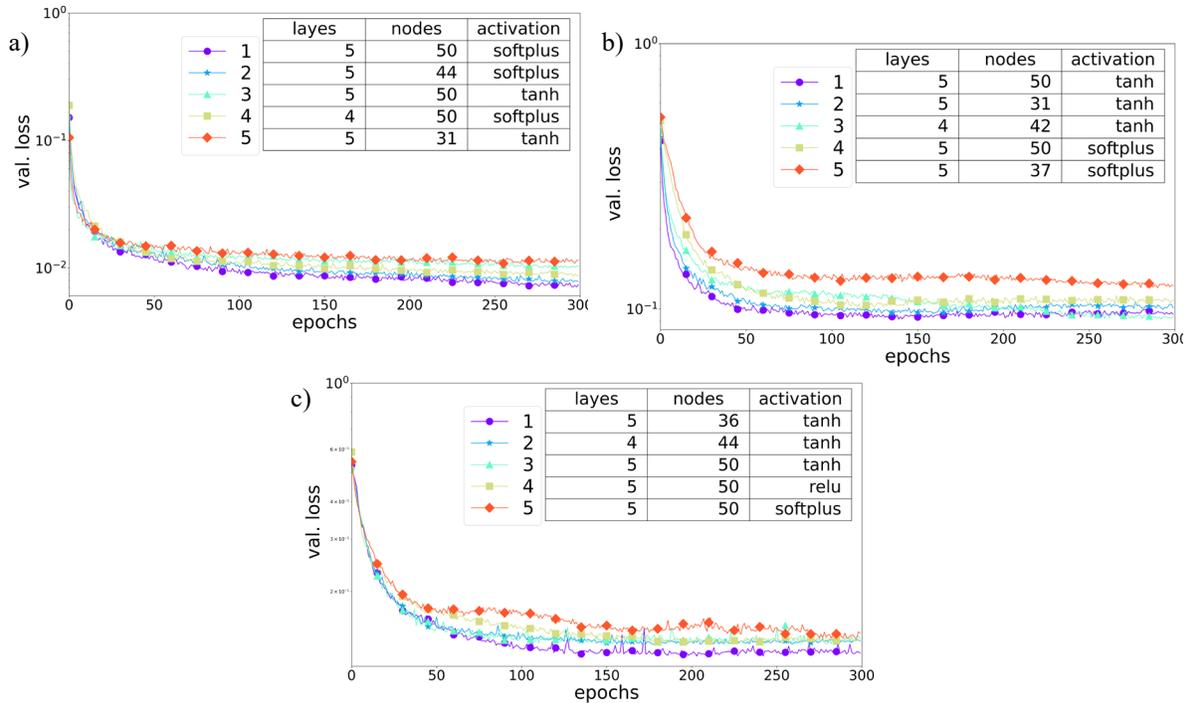
Fig. 3. Validation losses of the best five hyperparameter sets ranked by the automatic tuner: a) ANN $\epsilon$  with single network structure, b) ANN $\sigma$  with multiple network structure, c) PINN $\sigma$  with multiple network structure.
