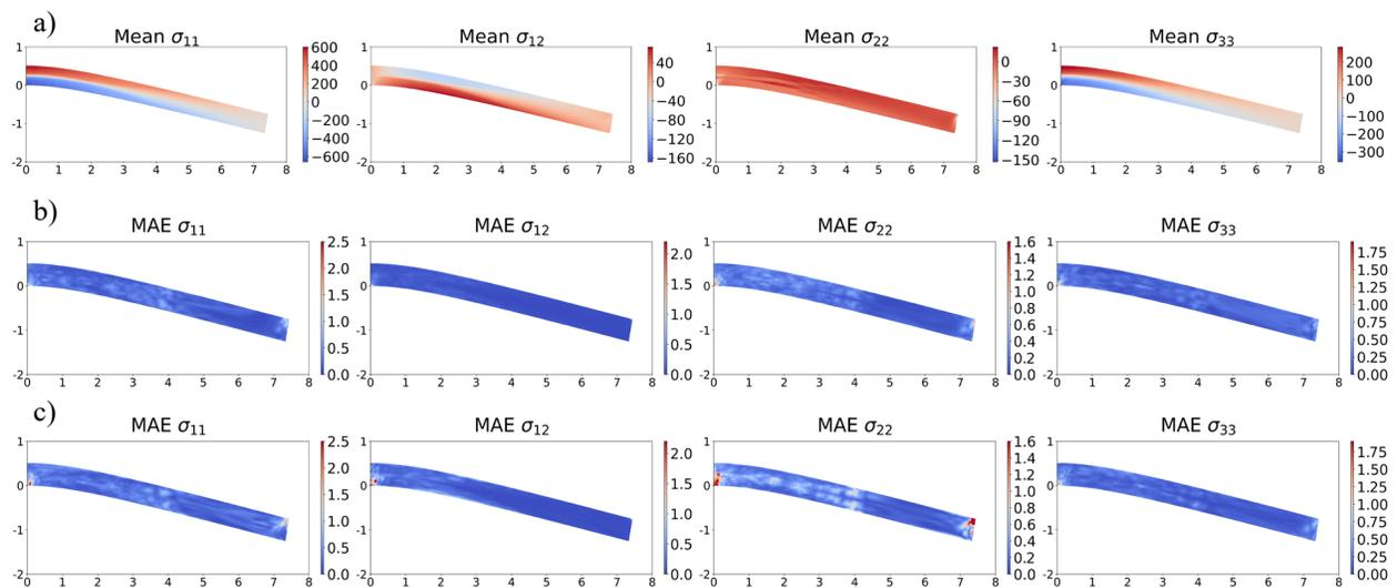
Fig. 6. a) Mean field of the stress, b) mean absolute error of  $ANN\sigma$ , and c)  $PINN\sigma$  for a third of the loading step.
