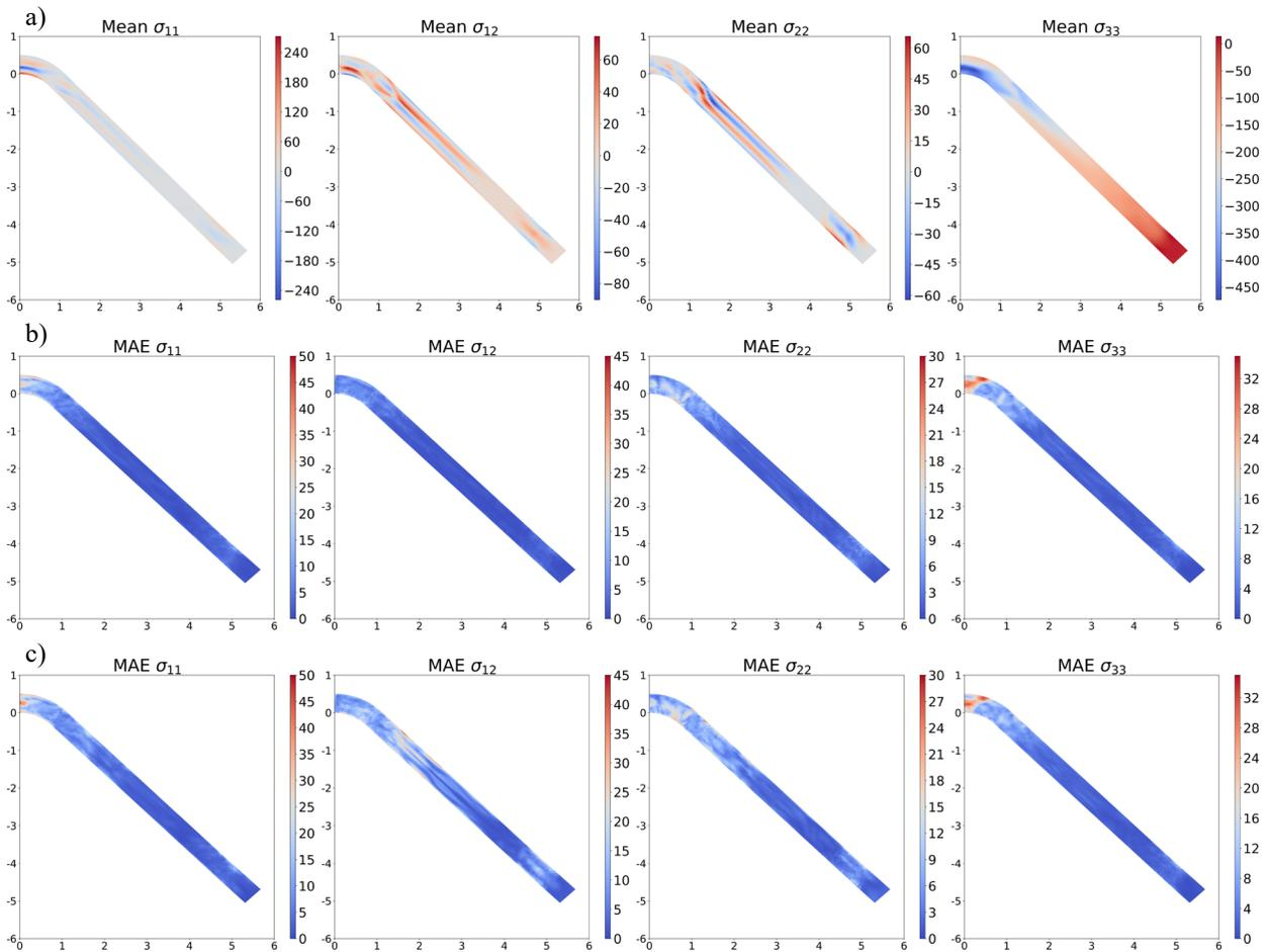
Fig. 5. a) Mean field of the stress, b) mean absolute error of ANN $\sigma$ , and c) mean absolute error PINN $\sigma$  for the loading-unloading cycle.
