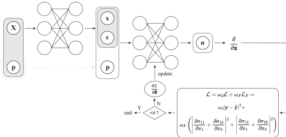
Fig. 1. Schematic representation of the sequential surrogate model; the  $\mathbf{p}$  vector contains the process variables. In the grey boxes are the inputs and outputs of the first surrogate model, while in the white boxes are the inputs and outputs of the second surrogate model.
