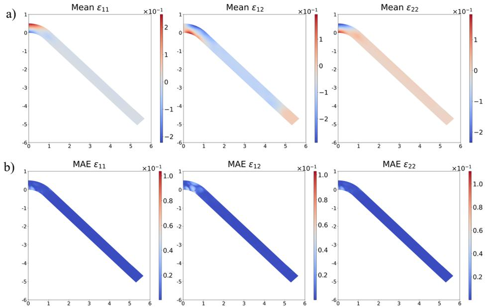
Fig. 4. a) Mean field of the strain and b) mean absolute error of the strain for the complete loading-unloading cycle.
