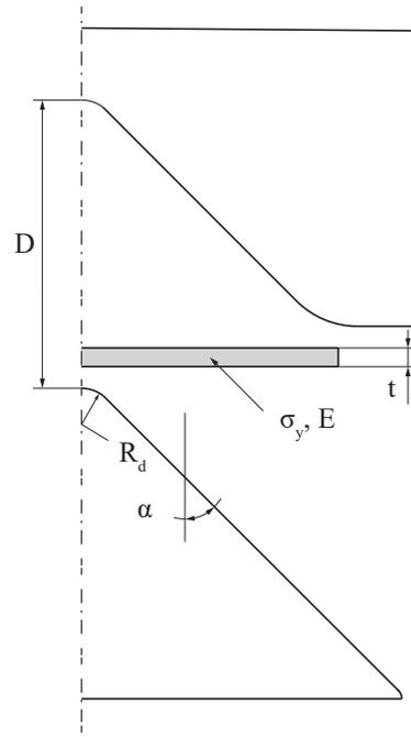
Fig. 2. 2D representation of the V-bending process implemented in the FE solver.
