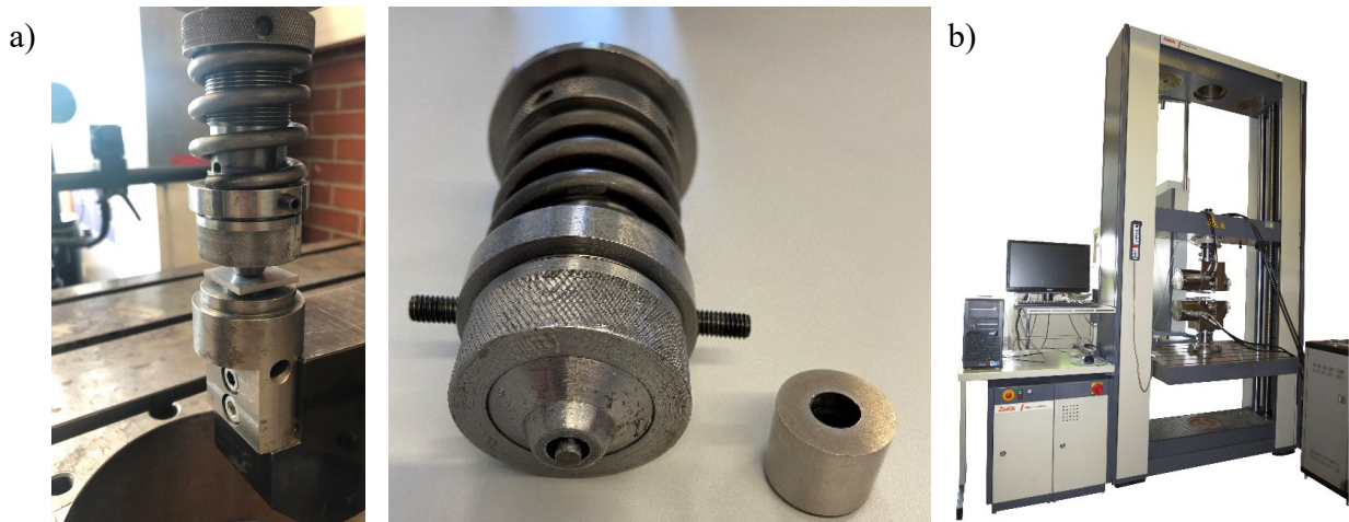
Fig. 2: Experimental setup of the punch indentation test
