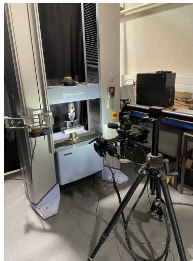
Fig. 2 - Shimadzu and GOM ARAMIS setup, with die, punch, and test specimen in place
