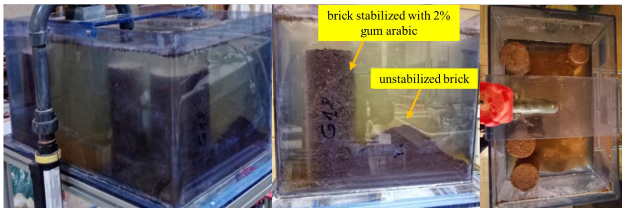
Fig.11: Cylindrical samples of clay-gum arabic mix immersed in water
