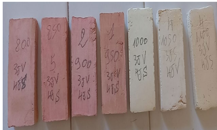
Figure 10: sintered bricks at different temperatures
