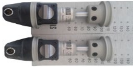
Figure 4 : Longitudinal displacement measuring device (extensometers)
