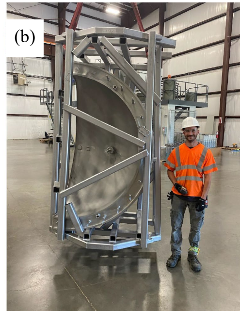
Figure 9. HIPed 1/2 top head (a) after powder filling and (b) in the support structure
