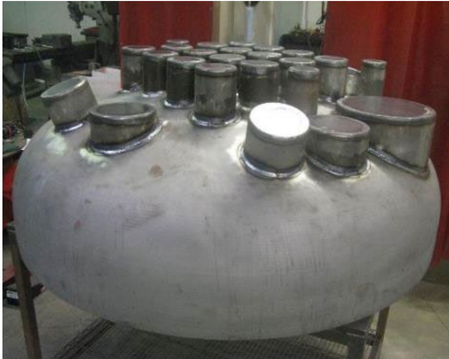
Figure 4. Welded capsule for 44% Top Head
