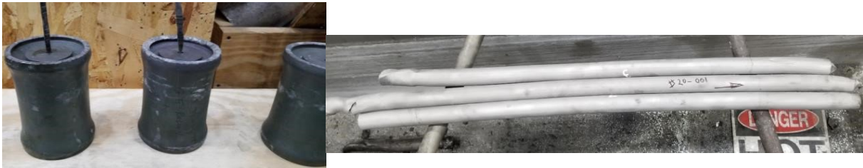
Figure 6: Three HIP billets and resultant extruded bars produced at different extrusion temperatures.
