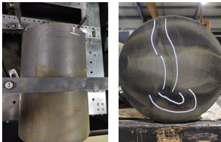
Figure 3. The stresses introduced by the heat treatment cause the MM 1.3344 bar to crack during EDM.
