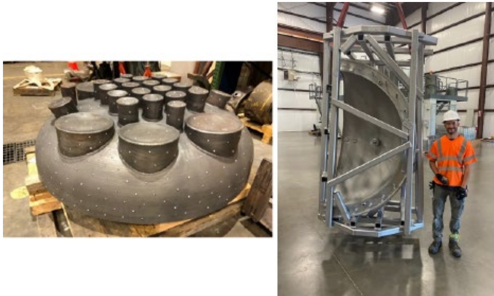
Figure 5. Scaling of large components such as a reactor head may take several iterations to reach acceptable dimensional and property requirements. A 44% upper head and one-half of a 67% upper head were manufactured under a large US DOE project [16].
