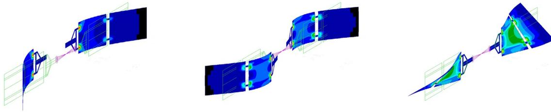
Fig. 2: Modal Strain Energy (MSE) map. From left to right, 1<sup>st</sup> mode, 2<sup>nd</sup> mode, 3<sup>rd</sup> mode
