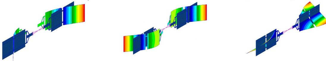
Fig. 1: Modal shapes. From left to right, 1<sup>st</sup> mode: 0.97 Hz, 2<sup>nd</sup> mode: 1.58 Hz, 3<sup>rd</sup> mode: 3.27 Hz
