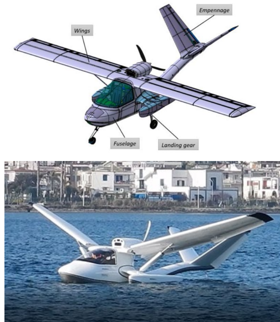
Fig. 2. Seagull: (top) sketch and (bottom) picture of the prototype in marine configuration
