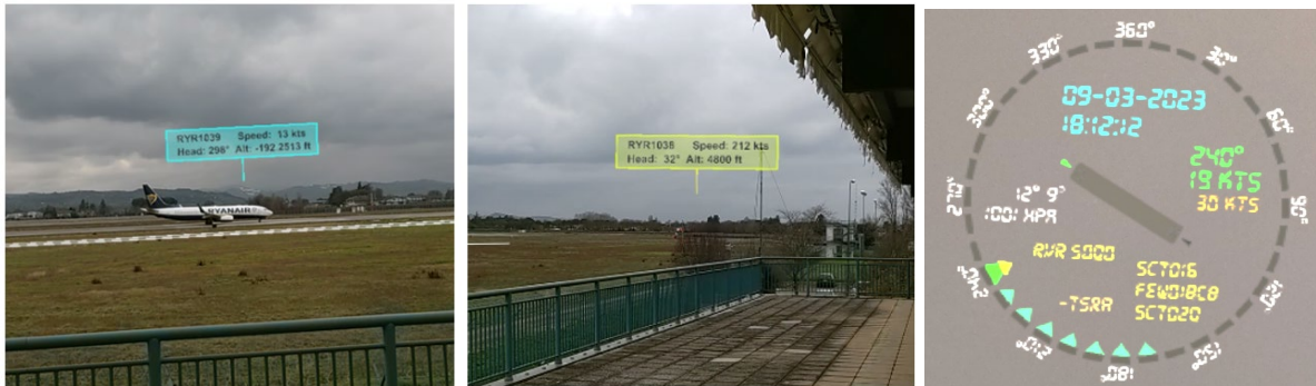
Figure 3. Tracking Labels visualization with runway overlay, colour coding, and weather interface
