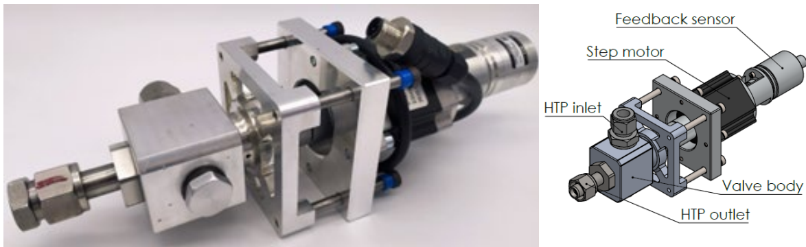
Fig 6. Moon Drone 400 N Main Engine Flow Control Valve
