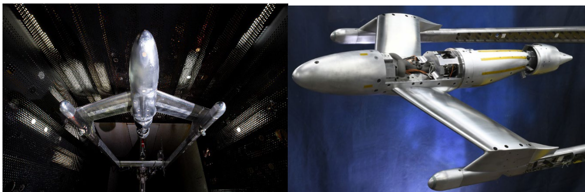
Figure 3: SUBLIME BLI360 configuration in wind tunnel
