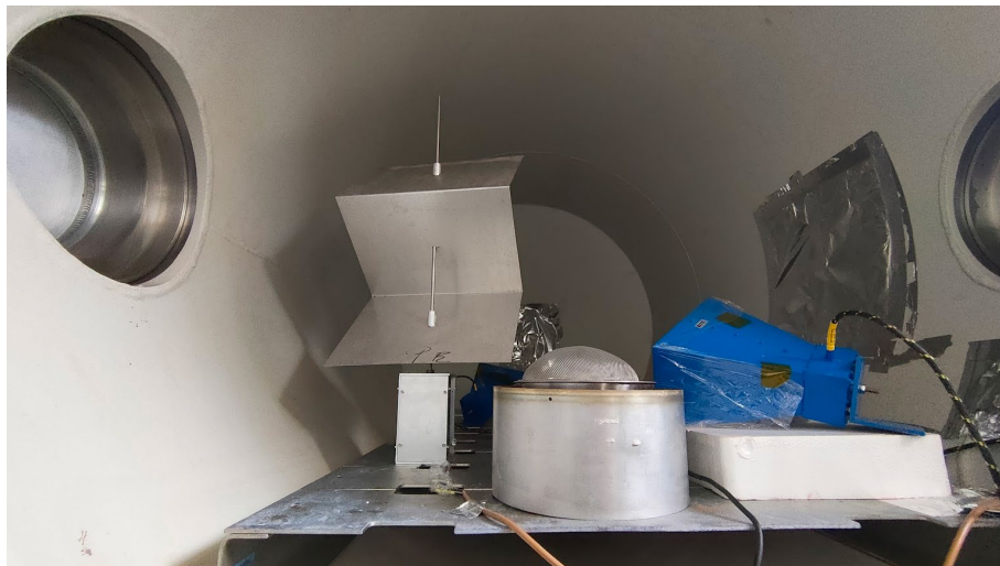
Fig.1. Inner view of the reverberation chamber for microwave characterization arranged by adapting the Space Environment Simulator of the Aerospace Systems Laboratory @ DIAEE – Sapienza Univ. of Rome.
