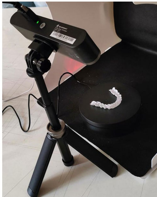
Figure 2 - Setup for acquisition of aligner Point cloud captured by Revopoint POP 2 scanner
