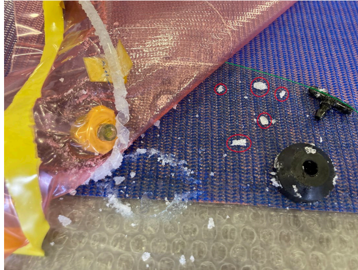
Fig.°2 – Clots in the connector circled in red
