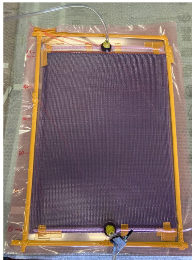
Fig.°1 – Experimental set-up for the infusion process
