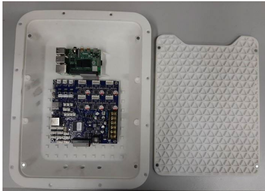
Fig. 4 Side case containing Duet 3 motherboard and Raspberry Pi 4.
