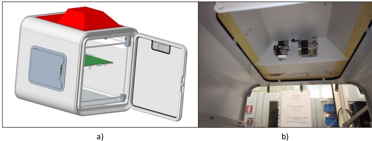
Fig. 3 New roof cover design: (a) CAD external view and (b) extruder fixing seat
