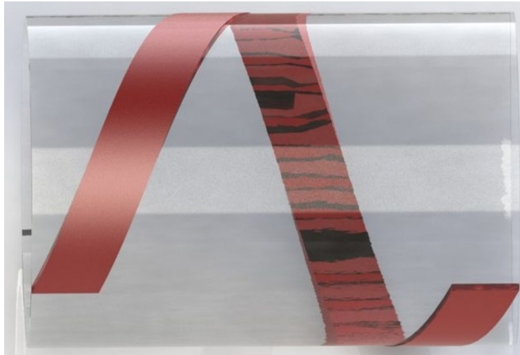
Fig. 2. Diagram of the method of heating the element (for better illustration, the pipe has been presented as transparent)
