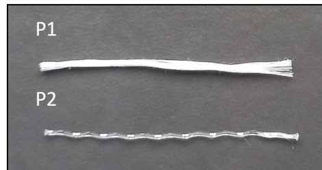
Fig. 1. Polypropylene fibers used in the tests (P1 fiber at the top, P2 at the bottom) [own study].
