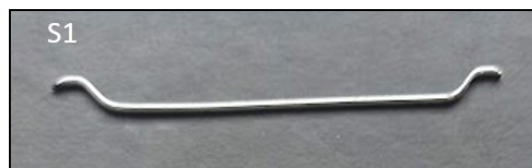
Fig. 2. Steel fibers used in the tests (S1 fiber) [own study].
