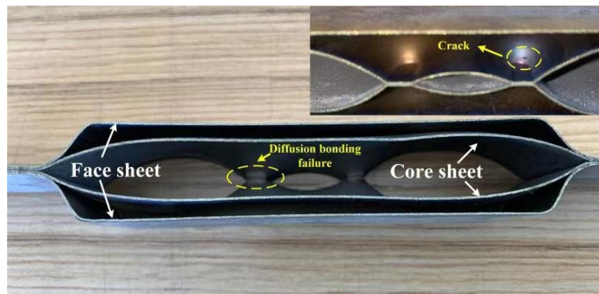
Fig. 5 Defects in four-layer structure components
