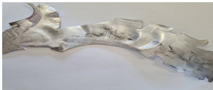
Fig.3. Laminated aluminum composite 5083/2024 after warm accumulative roll bonding (cycle 2)
