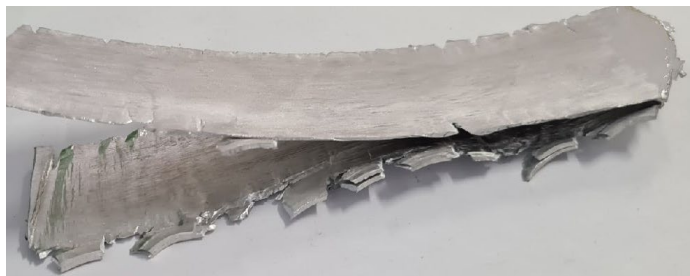
Fig.2. Laminated aluminum composite 5083/2024 after cold accumulative roll bonding (cycle 2)
