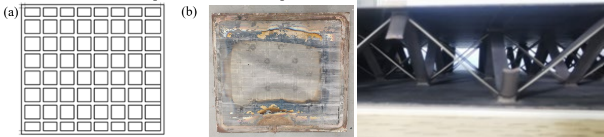
Fig. 3 The processed core sheet (a) and formed lattice structure (b)
