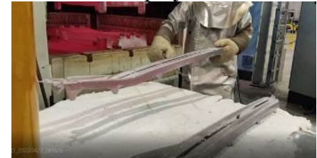
Fig15: Ti6242 production on 1.8x1.5 Press
