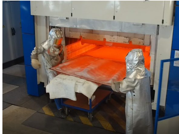
Fig 10: High-temperature SPF blank extraction at 920°C
