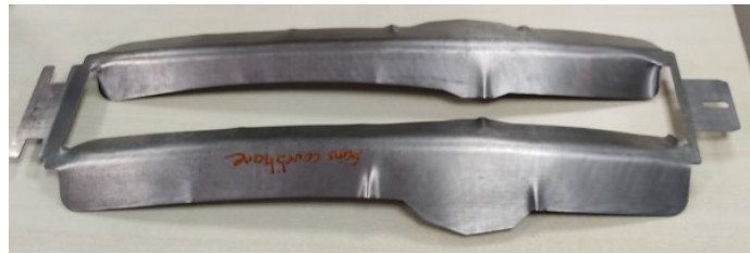
Fig 7: LAUAK studies with AUTOFORM to predict and localize critical zones (left) compared to real part trials (above).
