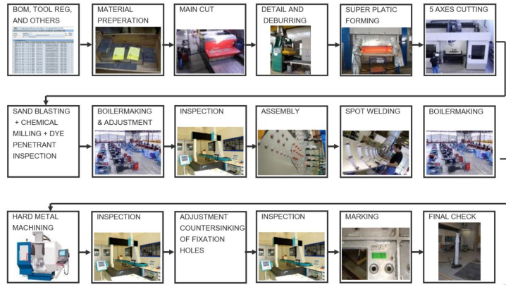
Fig 19 : Full production workflow of Heat Exchanger Cover
