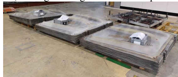
Fig 11 : Example batch of SPF formed blanks ready to be transferred to next operations (i.e. : Laser 3D Trimming)
