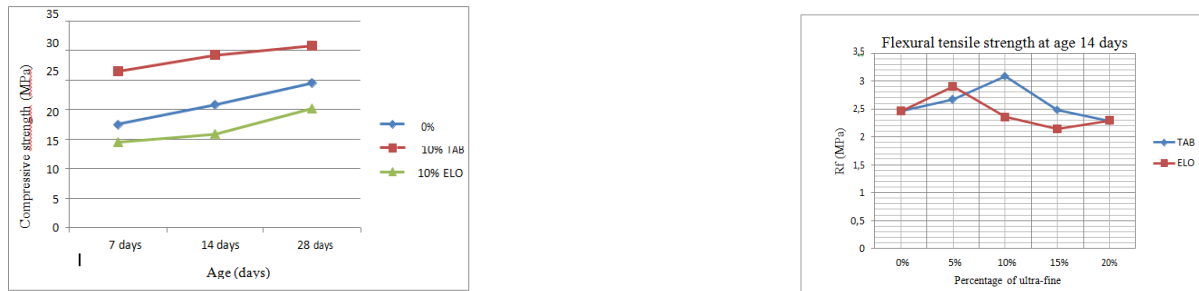
Fig. 14 Variation of compressive strength as a function of age of mortars containing 10% of ultras fines (TAB and ELO)
