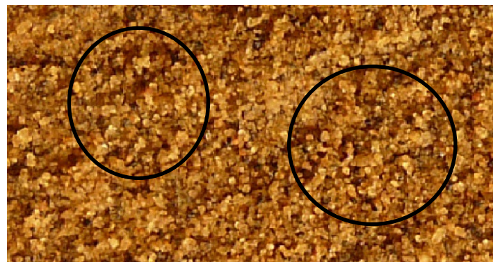
Fig 4. Digital image for the upper surface of a 95% sand and 5% bentonite liner leached by biofuel under a pressure of 100 kPa (cracks are showed in circles)
