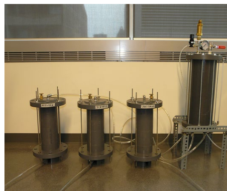
Fig.2. Column leaching test cells with pressure vessel setup
