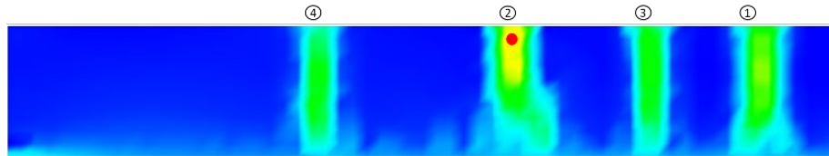
Fig. 6: Cracking patterns and marked sequences for wall with L/H 12
