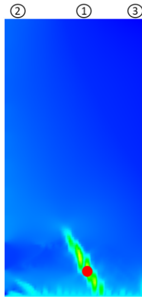
Fig. 10: Cracking patterns and marked sequences for wall with L/H 1
