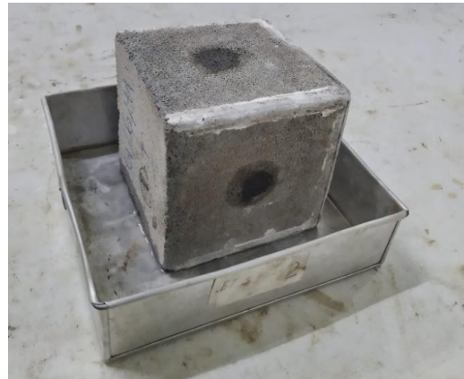
Figure 3. Initial Rate of Water Absorption (IRA) test
