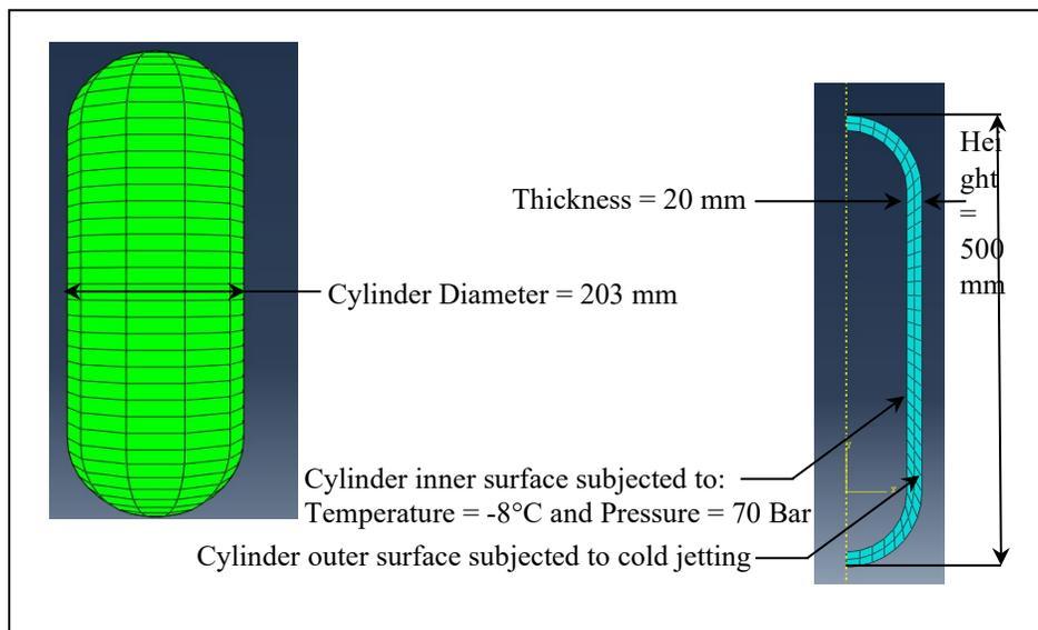
*Fig 4: Conceived pressure vessel axisymmetric model geometry and boundary conditions.*
