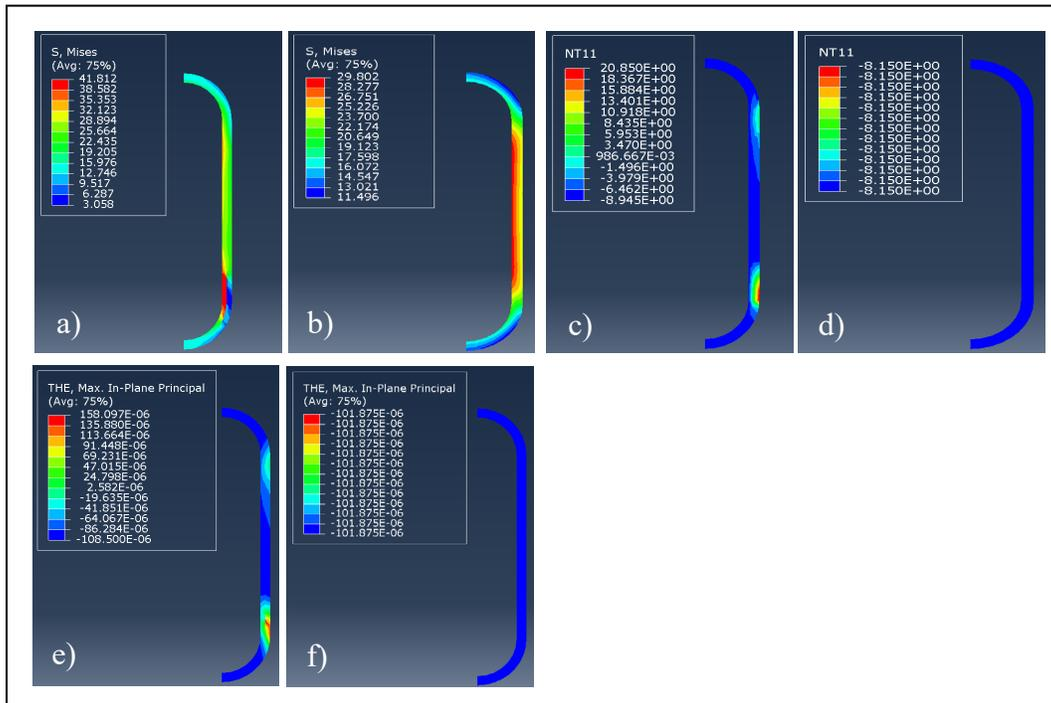
Fig 5: Von-Mises stresses (a, b), nodal temperatures (c, d) and thermal strains (e, f) profiles on pressure vessel with and without considering cold jetting effects, respectively.
