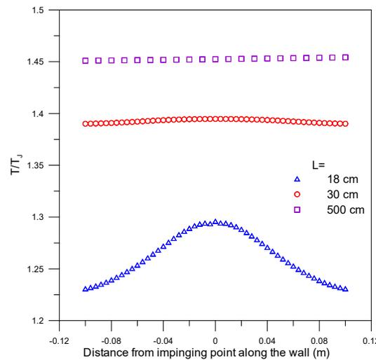
Fig. 3: Temperature Distribution along the Adjacent Wall when the inside Wall Temperature=265K
