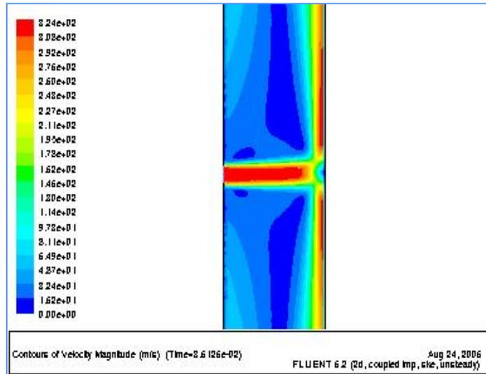
*Fig. 1: Velocity contours of jet impingement*
