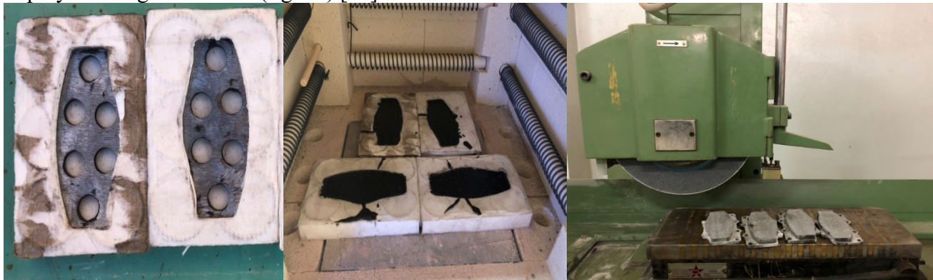
Figure 11. Brake pad backing plate. Figure 12. Polymerization Figure 13. Grinding of brake pads
