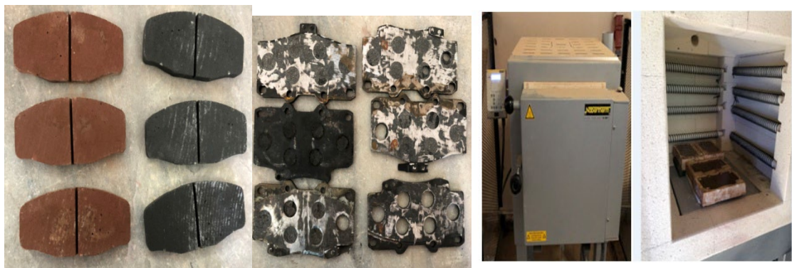
Figure 5. Brake pad linings. Figure 6. Base or backing plate. Figure 7. Polymerization oven..
