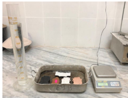
Figure 14. Capillary absorption test
