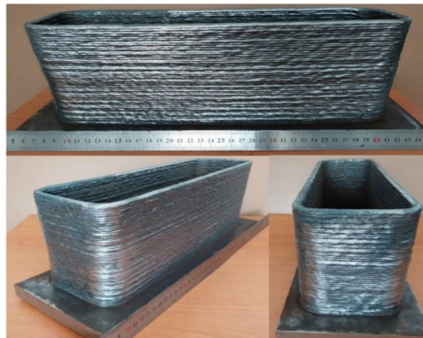
fig 14 – Real world example of fabricated part (WAAM)
