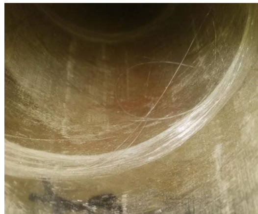
Fig 7: Morphology of failure along the fiber direction.
