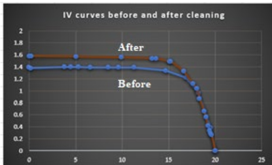
Figure 4 I-V curve for a 30-Watt solar panel before and after cleaning
