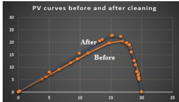
Figure 5 P-V curve for a 30-Watt solar panel before and after cleaning
