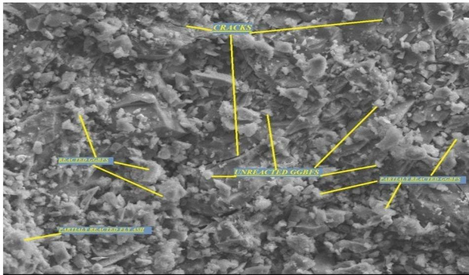
Fig. 5. Microstructural morphology of mix G-S-0.5
