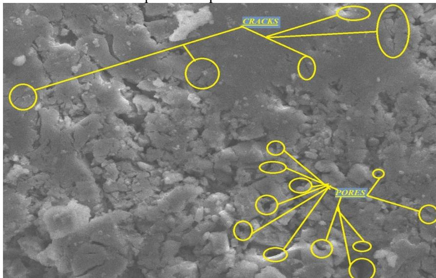
Fig. 4. Microstructural morphology of mix G-S-0.5
