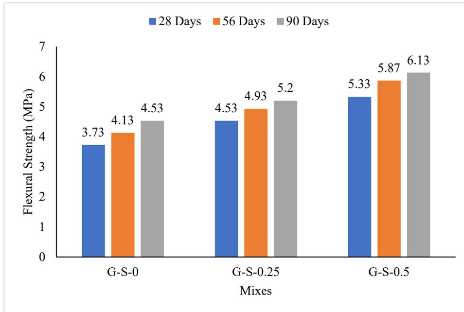
Fig. 3. Flexural Strength of SFRGPC
