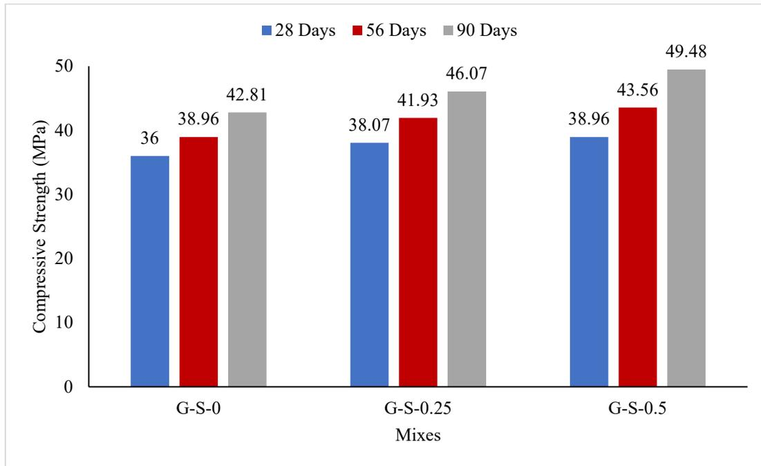
Fig. 1. Compressive Strength of SFRGPC
