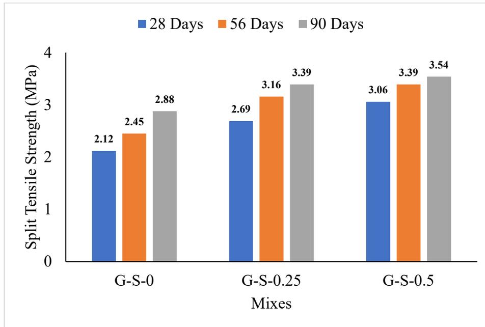
Fig. 2. Split Tensile Strength of SFRGPC
