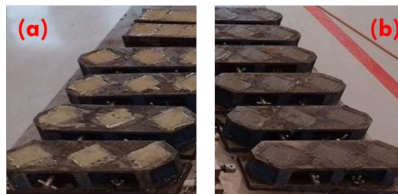
Fig. 4 Visual inspection of fresh mortar: (a) bleeding sign in M4-1.5% and (b) non-bleeding in typical mortar prepared with \leq 1\% of AG.
